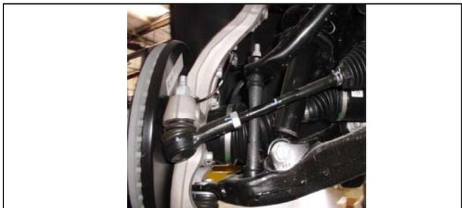
Reinstall the tie-rod using a 21mm socket. Reinstall the sway bar end links using a 13mm socket for the bottom and a 15mm socket for the top.
