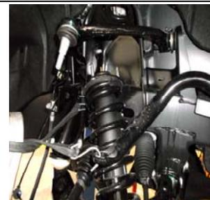
10. DO NOT over extend the cv-axle joints, doing so will damage/ break them. Lift the sway bar out of the way, then remove the strut from vehicle.
