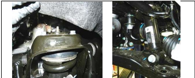
Remove the spring compressor. Install the top of the strut first using the supplied silver 10mm x 1.25 nuts and a 14mm wrench. Leave the nuts loose. Install the lower strut to the lower control arm using the factory bolt and a 21mm socket. Torque top nuts.
