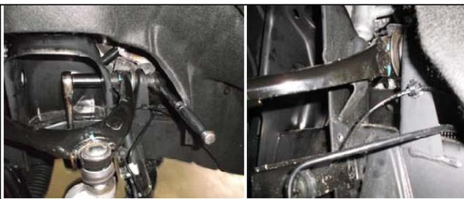
11. Loosen the upper control arm using a 13/16" socket and wrench. Let it rest on the droop stop, then retighten the upper control arm and torque it down to 90ft lbs. Loosening the lower control arms may be needed as well.
