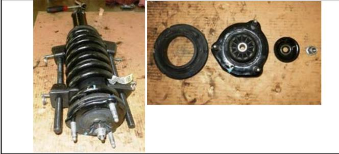
Once spring tension is off of the nut, remove the spring hat with a 15mm (nut) and 6mm wrench (shaft end). Remove the top hat and rubber isolator.
