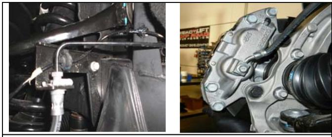
Reinstall the brake line brackets to the frame using a 13mm socket. You may need to lightly bend the brake line brackets to clear the upper control arm when at full droop. Reinstall the brake calipers to the rotors using a 18mm socket.
