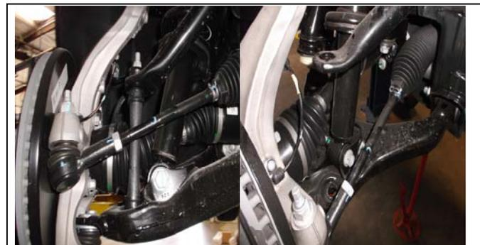
4. Remove the sway bar end links from the vehicle. Using a 15mm socket on top and a 13 mm socket on bottom.
