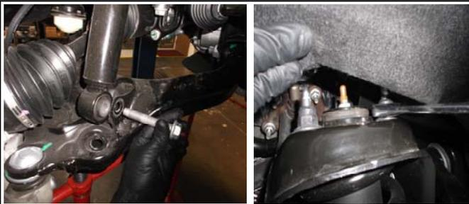
9. Loosen the lower control arms at the frame using a 24mm socket. Unbolt the strut from the lower control arm using a 21mm socket, then unbolt the top of the strut using a 18mm wrench.
