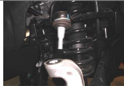
8. Separate the upper control arm from the steering knuckle using an 18mm socket. **Note: the upper control arm will be under tension.**
