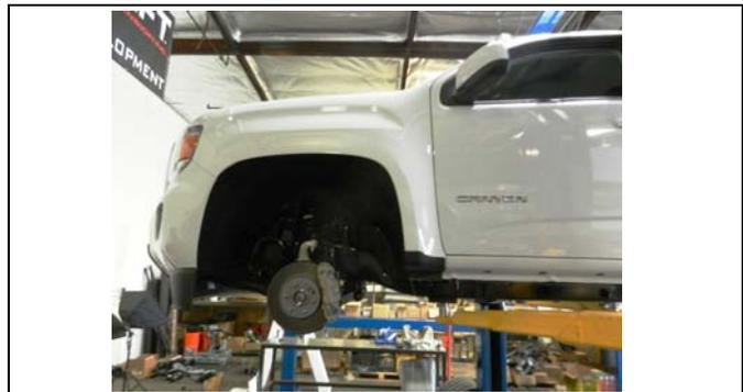
2. Lift the vehicle by the frame. Then remove the wheels using a 22mm socket.
