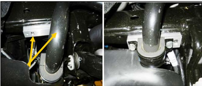
Install the sway bar offset spacers to the frame using the factory 10mm bolts. Install the sway bar to the offset spacer using the provided 10mm x 1.5 x 20mm bolts and a 14mm socket.
