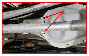
Remove the (2) middle bolts on the driver side differential cover and discard. Install the differential ID tag on the drivers side using the factory hardware.
