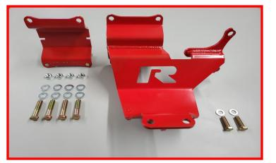
Install the center stabilizer bracket using the supplied 3/8" x 1-1/4" hex head bolts and 3/8" flat washers. Tighten bolts enough to secure the main body to the passenger side of the differential but do not tighten completely at this time.
