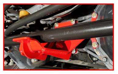
Using the supplied 7/16''x 2'' long Hex Head Bolts, 7/16" flat washers and 7/16" top lock nuts, install the rear axle clam shell to the center stabilizer bracket, clamping both around the axle tube.
