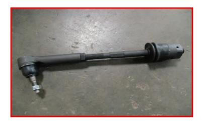
Install the assembly to the center link using a drop of thread locker on the inner tie rod end.
