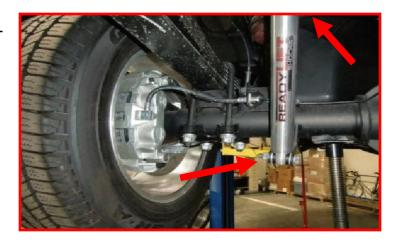
Remove the ABS harness clips from the axle to create slack.
