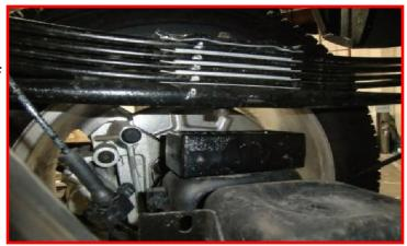
Install the provided u-bolts and hardware. Only snug the u-bolts up enough to hold the axle in place. Repeat all steps on the passenger side. Reattach the ABS harness clip to the axle. You may need unclip the clip and move the ABS down through the upper frame clip for clearance.
