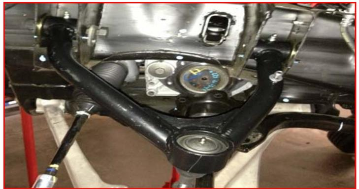
Raise the lower control arm and install the lower strut using the **factory hardware**. Torque to **45 ft-lbs**.
