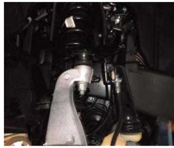
14. Reinstall the upper control arm into the steering knuckle using an 18mm socket. Torque down.
