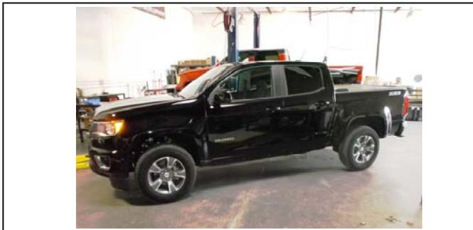
1. Put the vehicle onto level ground. Measure from the ground to the center of the fender well at all four wheels. Record the data in the space provided on page 2.
