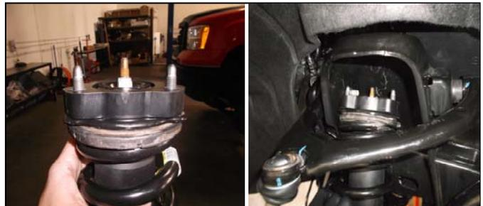
12. Add the spacer to the strut, put thread locker on the studs, then reinstall the strut into the vehicle. Use the provided hardware to mount the top of the strut with a 14mm wrench.
