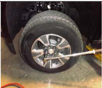
19. Reinstall the wheels using a 22mm socket, lower the vehicle to the ground and torque the lug nuts to 100 ft lbs.
