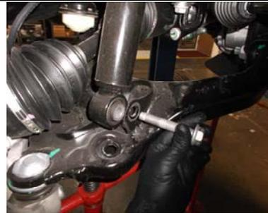
8. Loosen the lower control arms at the frame using a 24mm socket. Then unbolt the strut from the lower control arm using a 21mm socket.
