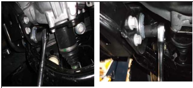
20. With vehicle on the ground, torque the lower control arms down using a 24mm socket. Double check all work performed on the vehicle. Then immediately have the vehicle aligned.
