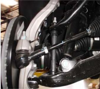
17. Reinstall the sway bar end links using a 13mm socket for the bottom and a 15mm socket for the top.
