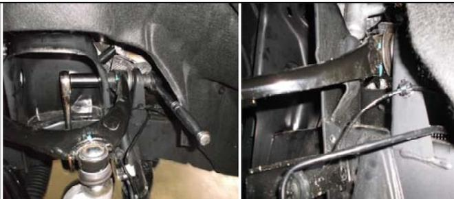
11. Loosen the upper control arm using a 13/16" socket and wrench. Let it rest on the droop stop, then retighten the upper control arm and torque it down to 90ft lbs.
