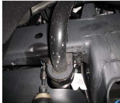
18. Retighten the sway bar at the frame using a 10mm socket.
