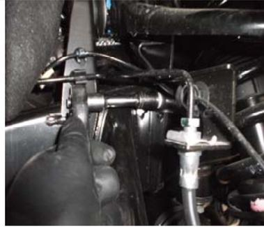
6. Remove the brake line bracket from the frame using a 13mm socket.
