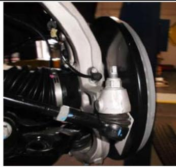
15. Reinstall the tie rods into the knuckle using a 21mm and 10mm wrench.
