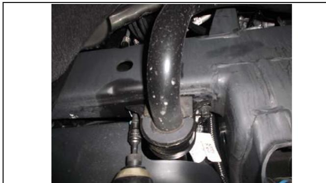
3. Loosen the factory sway bar at the frame using a 10mm socket.
