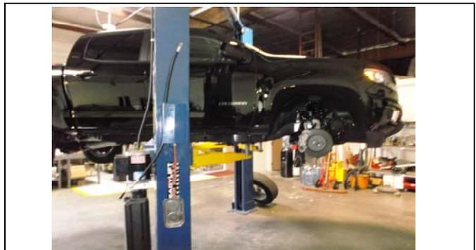
2. Lift the vehicle by the frame. Then remove the front wheels using a 22mm socket.
