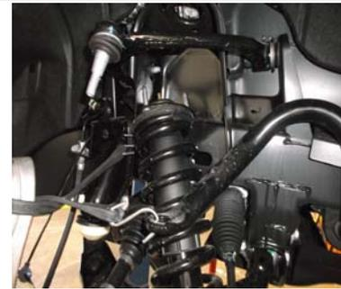
10. Lift the sway bar out of the way, then remove the strut from vehicle.
