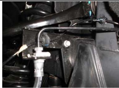
16. Reinstall the brake line brackets to the frame using a 13mm socket. You may need to lightly bend the brake line brackets to clear the upper control arm when at full droop.
