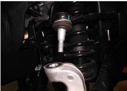
7. Separate the upper control arm from the steering knuckle using an 18mm socket. Note: the upper control arm will be under tension.
