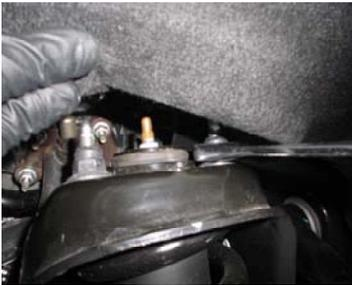
9. Unbolt the top of the strut using an 18mm wrench. Then drop the lower control arm to make clearance for the removal of the strut. Note: DO NOT over extend the cv-axle joints, doing so will damage/ break them.
