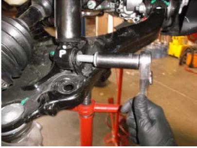
13. Raise the lower control arm and reinstall the bottom of the strut using a 21mm socket. Torque down.
