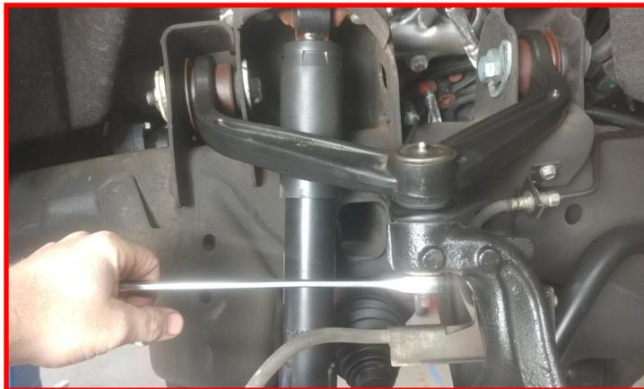
Strike the upper ball joint boss with a dead blow hammer to dislodge the taper. Mark the alignment cam's orientation and positions for reinstallation in a later step. Remove the upper control arm cam bolts.
