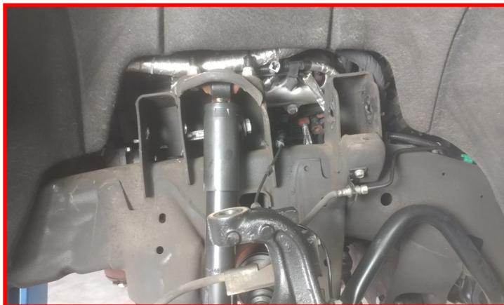
Install the ReadyLIFT upper control arm into the frame using the **factory cam bolts** in the same orientation as previously removed. Torque to **125 ft-lbs.**
