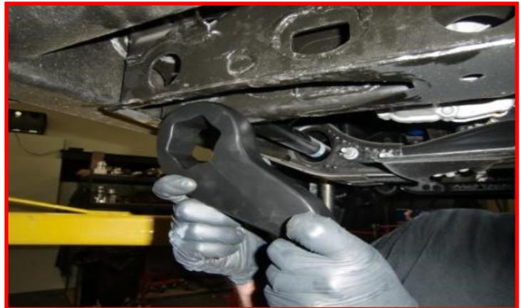
Use the torsion bar unloading tool, load the torsion bar enough to install the cross pin. Remove the torsion bar unloading tool. Install the keyway adjustment bolt using a dab of grease on the threads and tip. This is best to run up until 1/4" threads remain showing between the head of the bolt and the cross pin. This is a starting point for the last steps.
