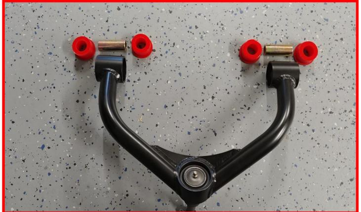
Install the ReadyLIFT appropriate side control arm to the frame rail using the factory hardware. Do not tighten at this time. To determine the correct side arm, there is a plugged hole on the back tube of the near the rearmost pivot.
