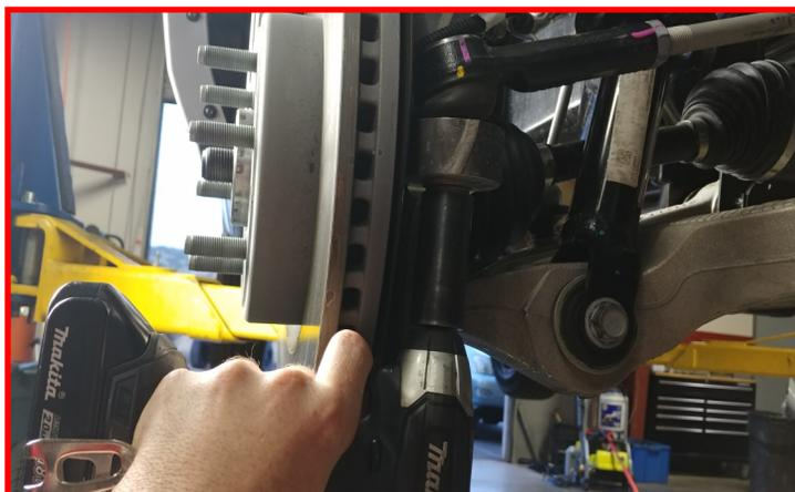
Strike the tie rod boss on the knuckle with a dead blow hammer to dislodge the taper.
