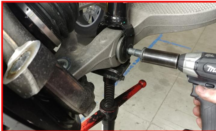
Attach the upper control arm ball joint to the knuckle using the provided hardware. Install the **nut spacer**, then the **castle nut**. Torque to **65 ft-lbs**. Install the provided **cotter pin**. Use a suitable grease gun, fill the upper ball joint with grease until the boot just starts to expand. Do not overfill. Typically 5 to 10 pumps of a hand held grease gun.
