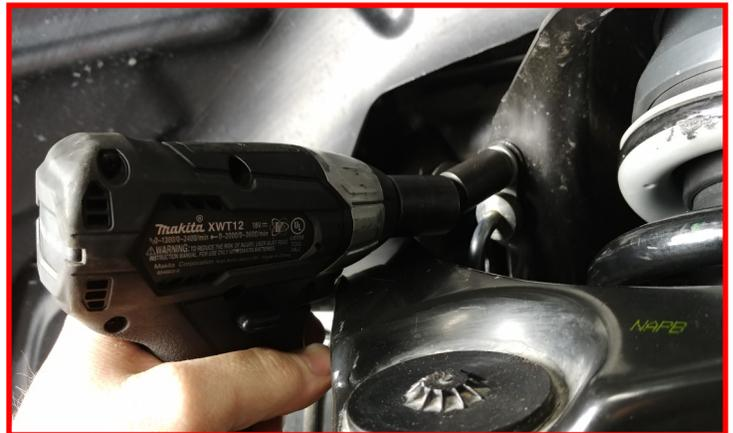
Remove the ABS wire harness from the upper control arm and frame rails. Cut the Christmas tree clip off the harness. Do not cut the ABS wire.
