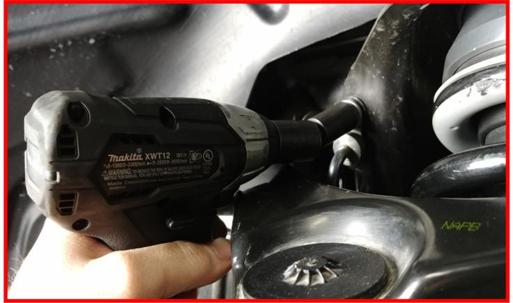
Install the sway bar to the frame rail using the **factory hardware**. Torque to **35 ft-lbs**.
