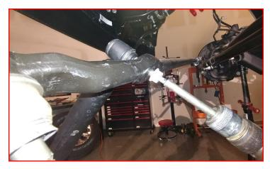
Remove the factory bump stop by grabbing and pulling it out of its mount using a twisting/pulling motion.
