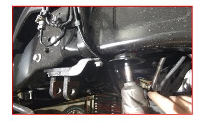
Install the ReadyLIFT bump stop extension to the frame by threading it into the existing bolt hole. Use a punch or similar tool in the holes of the mount and tighten. Install the bump stop mount to the extension using M8 nut and washer. Mark a line across the edge of the outer lip of the bump stop mount parallel to the frame.
