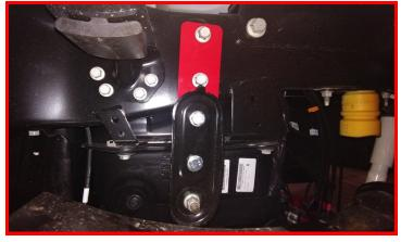
Install the provided extended rear shocks using factory hardware. Do not tighten at this time.
