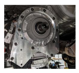
Re-install transfer case using the provide M10-1.5 x 35mm Hex Bolts. Using a star pattern, torque bolts to 50 ft-lbs.
