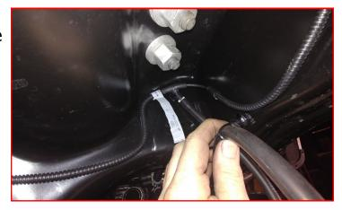
Remove the vacuum line clip from the passenger side engine cross member.
