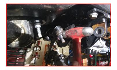
Remove the steering stabilizer from the frame.
