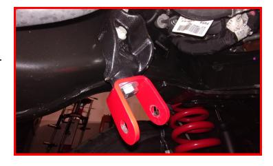
Install the ReadyLIFT steering stabilizer bracket to the tie rod using M12 x 55mm bolt, washers, cone adapter, and nut. Cone adapter will install from the bottom going up. Do not tighten at this time. The stabilizer must be test fit to establish the bracket's final orientation.
