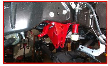
Install the track bar into the ReadyLIFT track bar mount using the factory hardware and the ReadyLIFT offset square washers. Ensure that the offset is closest to the passenger side. Do not tighten at this time.
