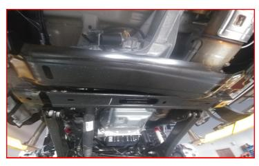
Support transfer case with jackstand near the output shaft. Remove factory cross member and discard. Retain the 4 factory bolts and nuts that hold the transfer case on the outsides.
