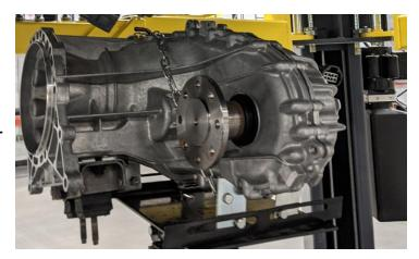
Install the ReadyLIFT Transfer Case Clocking Ring into the transmission using the provided M10 x 35mm socket cap bolts. Using a star pattern, torque bolts to 50 ft-lbs.
