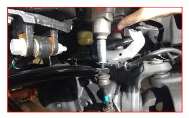
Remove the sway bar from the frame. Note orientation of the bar for reinstallation.
