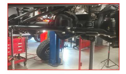
Remove the radius arms at the frame. Use the jack to rotate the axle up allowing the radius arms to drop out of the frame low enough to clear the ReadyLIFT radius arm drops.
