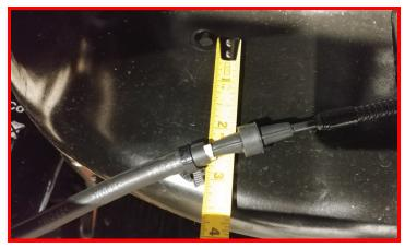
Locate the forward hole on the driver side spring mount on the bottom of the frame rail. Drill into frame rail using 3/8" drill bit. Install the differential vent line clip into the hole.
