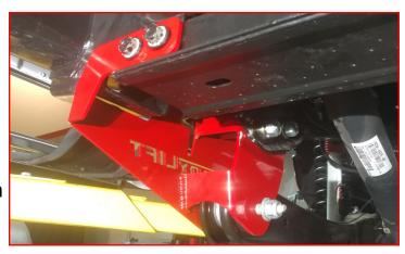
Remove the jacks from under the tie rod ends and place under the axle.
