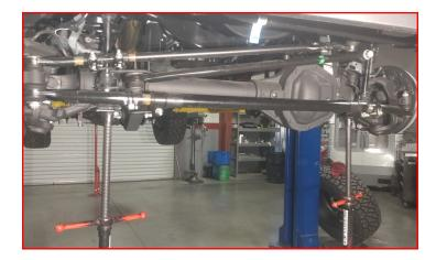
Remove the sway bar end links from the sway bar and axle.
