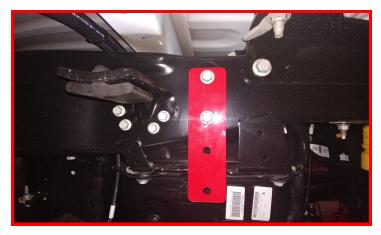
Install the factory sway bar bracket to the ReadyLIFT drop bracket using M12 x 35mm bolts, washers, and nuts. Torque to 45 ft-lbs.
