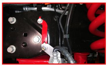
Passenger side: gently unbend the metal line until you can line up the ReadyLIFT bracket locking tang into the original bolt hole. Make sure to not kink the metal line. Install using factory hardware. Do not over tighten and strip the threads.
