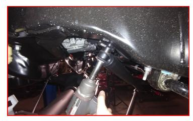
Remove the steering stabilizer nut from the drag link. Dislodge the taper to remove the steering stabilizer. Discard.
