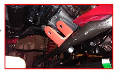
Install the steering stabilizer to the brackets using M12 x 70mm bolts, washers, and nuts. Mark the orientation of the brackets to the tie rod end and frame mount. Remove the stabilizer. Torque the mount hardware to 45 ft-lbs. Reinstall the steering stabilizer and torque hardware to 45 ft-lbs.
