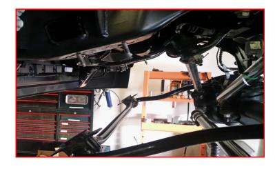
Remove the track bar at the track bar bracket. Let hang out of the way.
