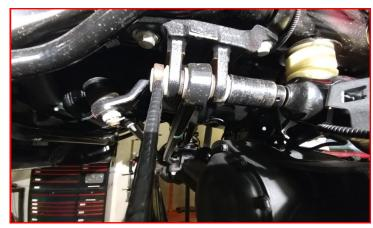
Remove the shock from the axle.
