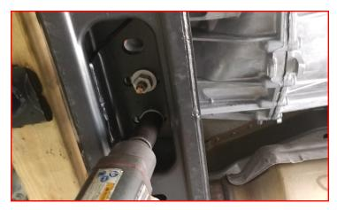
With the transfer case still supported, remove the front and rear drive shafts from the vehicle. Retain factory driveshafts and hardware. Unclip the wiring harness from the transfer case.
