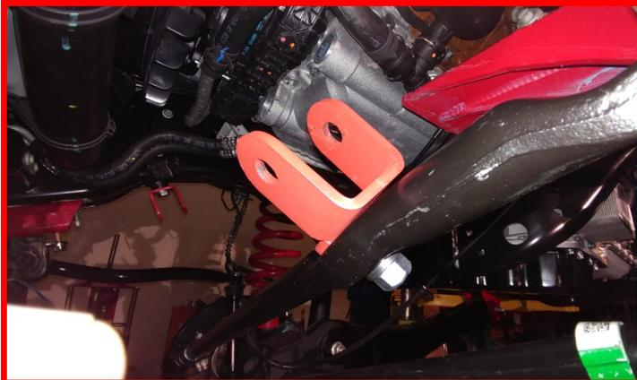
Install the steering stabilizer to the brackets using **M12 x 70mm bolts, washers, and nuts**. Mark the orientation of the brackets to the tie rod end and frame mount. Remove the stabilizer. Torque the mount hardware to **45 ft-lbs**. Reinstall the steering stabilizer and torque hardware to **45 ft-lbs**.
