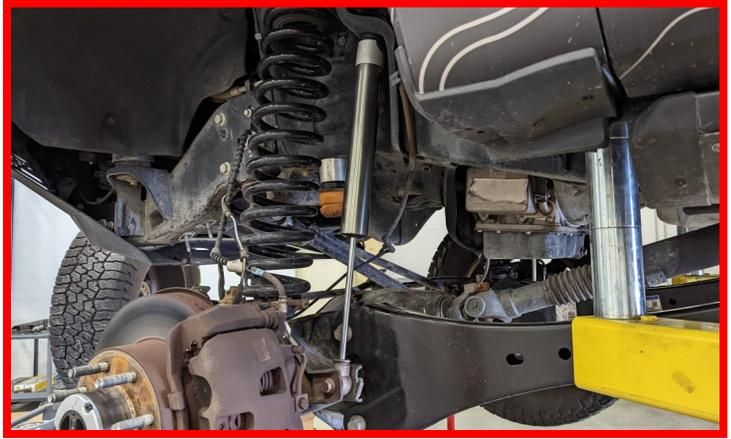
Make a mark 2.5" below the original vacuum line mount on the passenger side engine cross member. Drill a hole using 3/8" drill bit. DO NOT drill into the oil pan. Install the vacuum line clip into the newly drilled hole.
