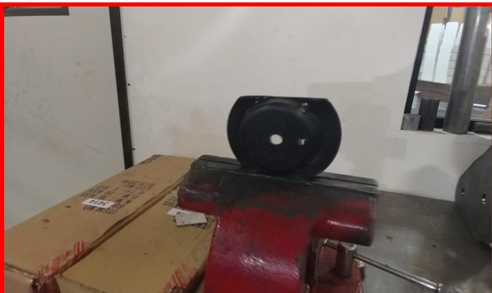
Re-install bump stop mount to the ReadyLIFT extension making sure the cut edge faces to the outside of the vehicle. Torque to 5 ft-lbs.
