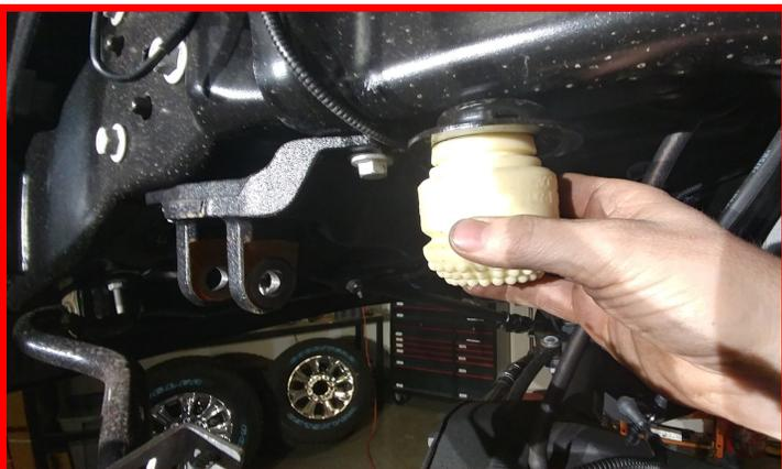
Mark a line across the edge of the outer lip of the bump stop mount parallel to the frame. Remove the bump stop mount from the frame.
