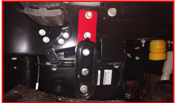
Install the factory sway bar bracket to the ReadyLIFT drop bracket using **M12 x 35mm bolts, washers, and nuts**. Torque to **45 ft-lbs**.
