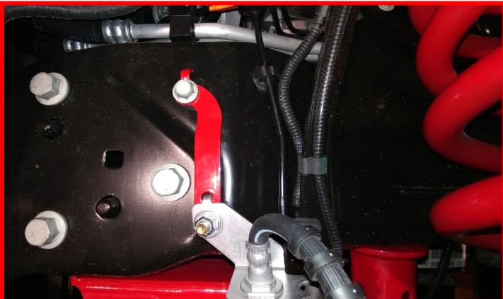
**Passenger side:** gently unbend the metal line until you can line up the ReadyLIFT bracket locking tang into the original bolt hole. Make sure to not kink the metal line. Install using **factory hardware**. Torque to **5 ft-lbs**. Do not over tighten and strip the threads.
