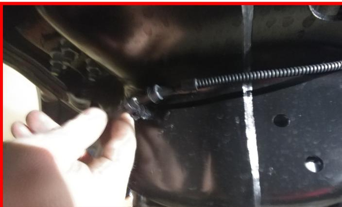
Mark the drive shaft to pinion orientation, then remove the drive shaft from the front differential. Tape the u joint caps to keep them from falling off / damage while working. Retain factory hardware.
