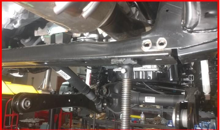
Install the ReadyLIFT radius arm drop bracket into the frame using **M18 x 130mm bolts, washers, crush sleeve, nuts and the factory cross member bolts**. Do not tighten at this time. Move the jack holding the cross member to the opposite side and repeat above steps.
