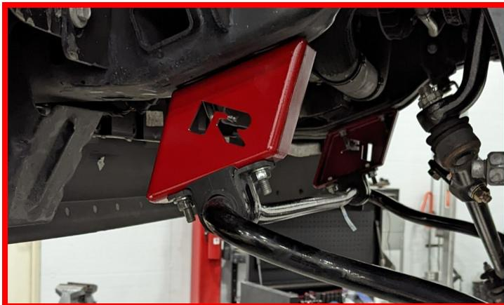
Install the front wheels. Lower the vehicle to the ground. Torque the lug nuts to the wheel manufacturers specs. Jounce the vehicle a few times to settle it to the new ride height. Install the front drive shaft using the **factory hardware with a drop of thread locker**. Torque to **26 ft-lbs**, then the upper shock hardware to **30 ft-lbs**, the lower shock hardware to **65 ft-lbs**, the radius arm hardware to **200 ft-lbs**, track bar at the bracket to **350 ft-lbs**.
