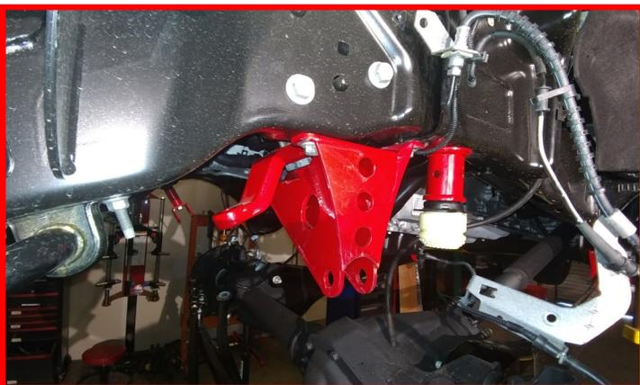
Install the factory isolator onto the ReadyLIFT springs, and then the springs onto the axle making sure to clock the dead end of the spring into the spring lock. Raise the axle enough to hold the springs into place.
