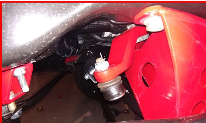
Install the ReadyLIFT steering stabilizer bracket to the frame using **M12 x 35mm bolt and washer**. Do not tighten until the stabilizer has been test fit so as to establish the brackets final orientation.
