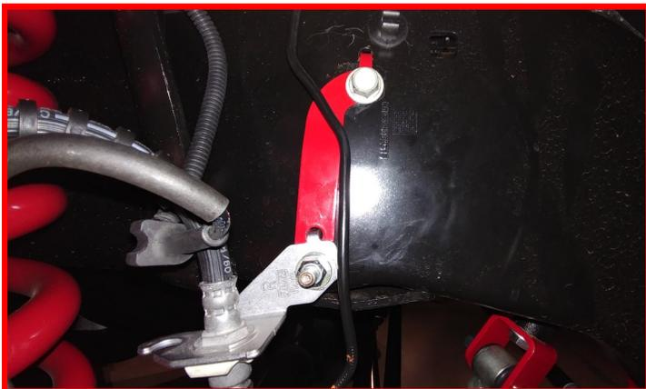
Install the ReadyLIFT sway bar brackets to the frame using **factory hardware**. Torque to **45 ft-lbs**.
