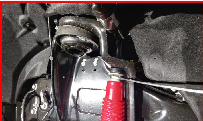
Remove the factory bump stop by grabbing and pulling it out of its mount using a twisting/pulling motion. Retain factory bump stop.
