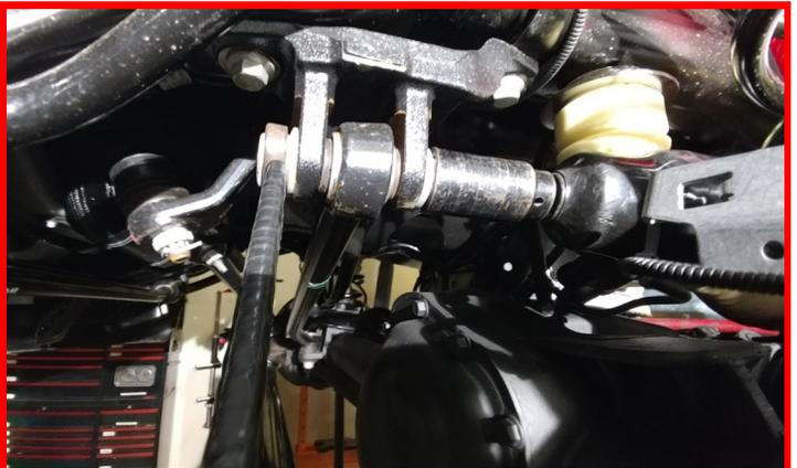
Remove the tie rod end at the pitman arm. Strike the pitman arm with a dead blow hammer to dislodge the taper. Retain factory hardware.
