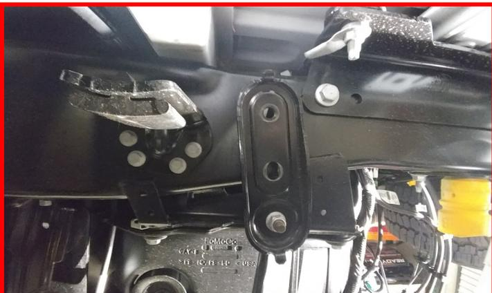
Support the axle with a suitable jack. Remove the rear shocks from the axle and frame. Retain factory hardware.
