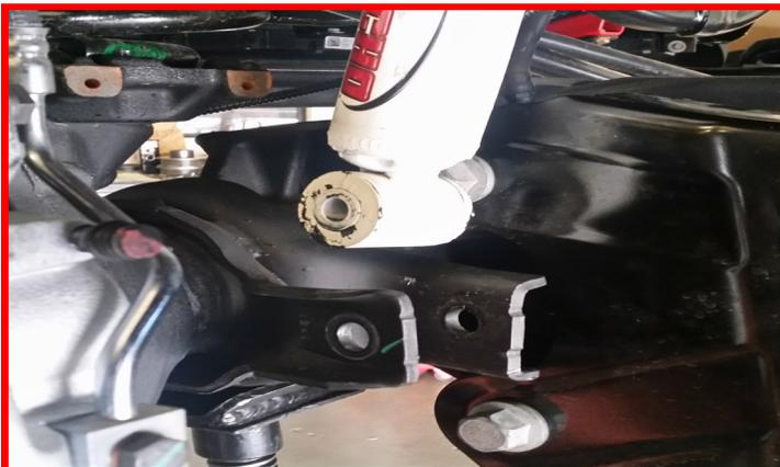
Lower the axle enough to remove the front springs. Remove the shock from the frame. Discard factory shocks and springs.
