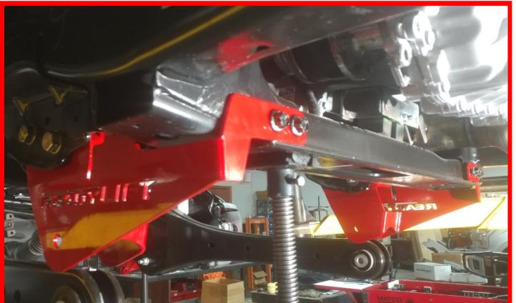
Rotate the axle by lowering the jacks under the tie rod ends until you can line up the radius arms into the ReadyLIFT drop brackets. Install using **factory hardware**. Do not tighten at this time. Torque the transmission cross member bolts to **40 ft-lbs**.
