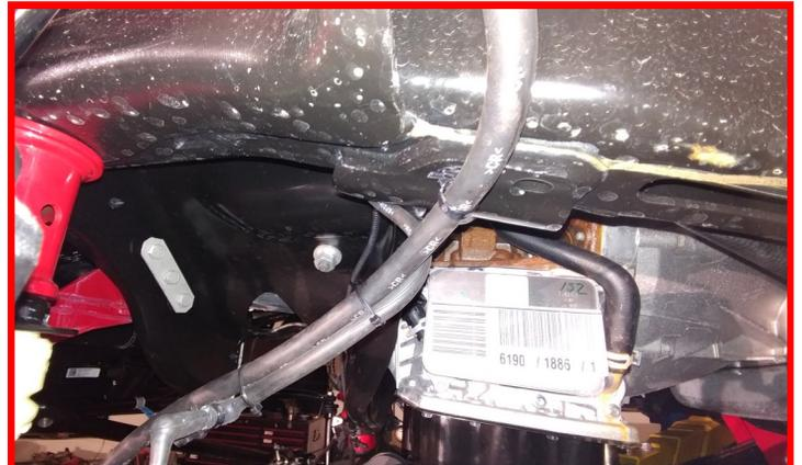
Install the ReadyLIFT brake line extensions to the factory brackets using **5/16" x 3/4" bolts, washers, and nuts**. Install bolts facing outwards.
