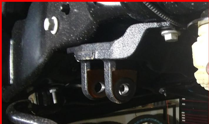
Remove the pitman arm nut. Using a pitman arm puller, remove the pitman arm from the gear box. Clean off any debris off the sector shaft. Coat the sector shaft splines with a light duty liquid based lubricant or oil.
