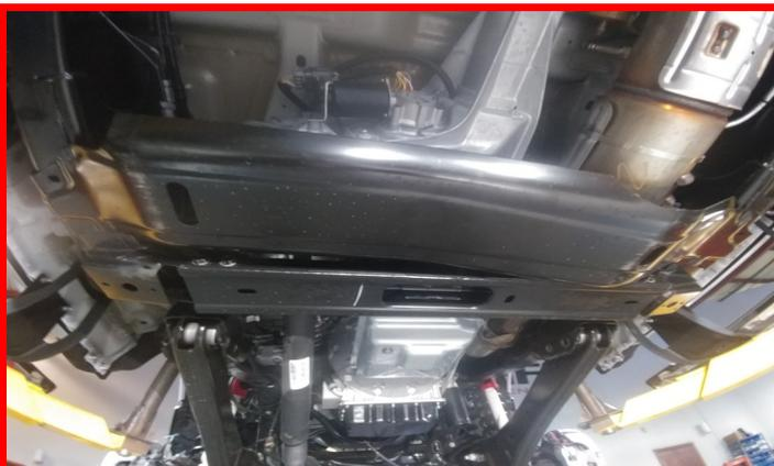
Leave the axle hanging from the shocks. Place a suitable jack under the tie rod ends close to the knuckles.
