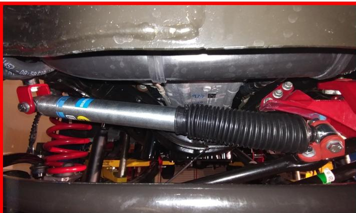
Install aftermarket front shock to the axle. Torque upper hardware to **35 ft-lbs**. Do not tighten lower hardware at this time.
