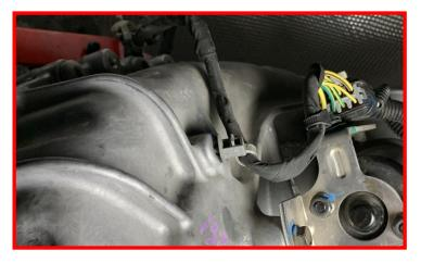
Install the transfer case harness retaining clip located on the top of the transfer case.
