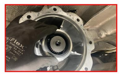
Install the transfer case. It may be necessary to rotate the shaft on the front of the transfer case to match the spline pattern for the back of the transmission.
