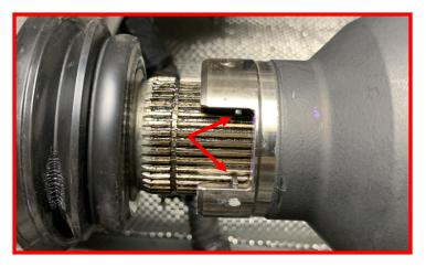
Mark the rear driveshaft to pinion flange location. Remove the rear driveshaft hardware from the flange. Let hang out of the way.
