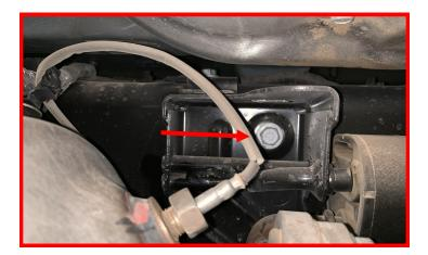
Remove the (2) Diesel Exhaust Fluid (DEF) tank crossmember exhaust hanger mounting bolts.
