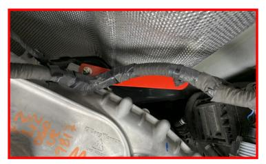
Install the transfer case shift solenoid connector.
