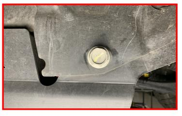
Remove the (4) transmission crossmember bolts and retain factory hardware.
