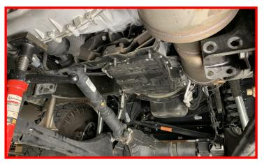
The transmission mount is attached with (4) bolts. Remove the (2) bolts located at the rear of the mount.
