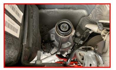
Install the rear driveshaft to the pinion flange lining up the previous marks using the factory hardware and thread locker.
