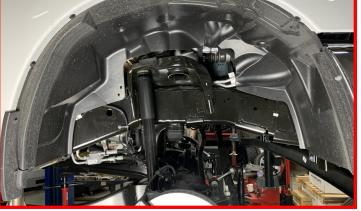
Install provided track bar drop bracket using factory hardware and provided M14 hardware.
