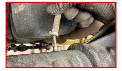
Install the provided rear shocks upper and lower mounting locations on both driver and passenger side using the factory hardware.
