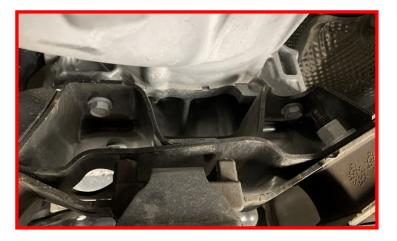
Tighten the transmission mount bolts.
