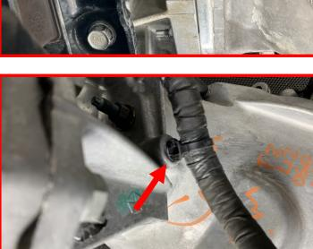
With the connector out of the way, install the connector relocation bracket using the provided M6 hardware.
