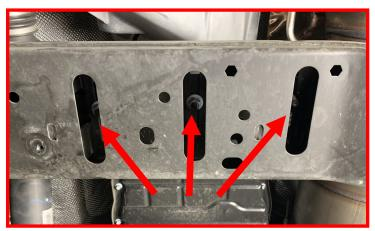
Remove the (3) transmission mounting nuts.
