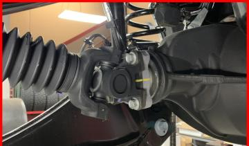
Rotate the axle to release radius arms from the mounting locations.
