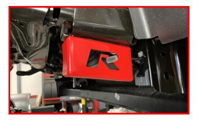
Install the sway bar to the drop brackets using the provided 7/16" hardware.
