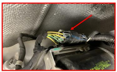
Remove the transfer case harness retaining clip on the rear of the transfer case.
