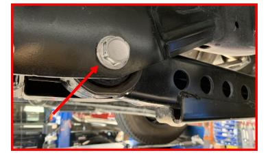
Mark the driveshaft to pinion location. Remove the front driveshaft from the axle. Let hang out of the way.
