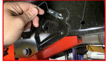
Tighten the provided 1/2" bolts first, ensure the drop bracket is resting flush against the frame rail when doing so.
