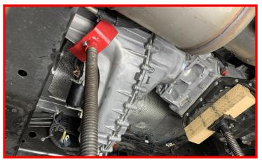
Install the transmission mount using the (4) factory bolts.
