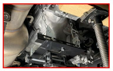
Remove the (8) transfer case mounting nuts.
