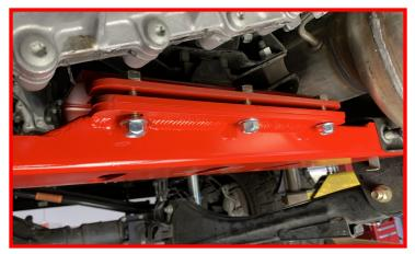
Install (3) provided M12 bolts, (3) locking nuts and, (6) flat washers through the front holes on the transmission mounting plate, mounting plate spacer and the transmission crossmember. Lower the transmission down on top of the mount.
