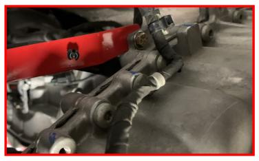
Using a suitable jack, support the transfer case again. Be sure to allow yourself ample room around the transfer case.
