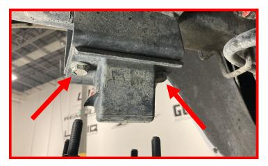
Install the provided bump stop extensions using the provided hardware.
