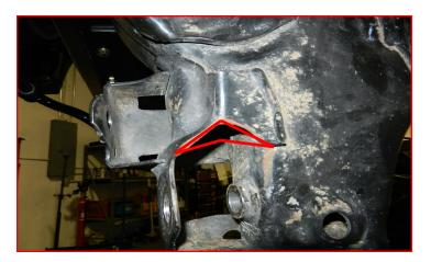
Torque the front cross member bolts to 200 ft-lbs, rear cross member bolts to 150 ft-lbs, 1/2" diff hardware to 95 ft-lbs, and M14 differential hardware to 80 ft-lbs.
