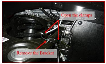
Remove the brake line brackets from the frame and knuckle.
