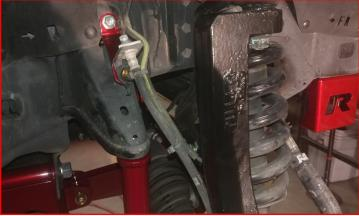
Run the ABS wire over the upper control arm. Install the ABS sensor and bracket to the knuckle using factory hardware. Turn the knuckle until it hits the turn stop. Using tie wraps, secure the ABS wire along the brake line up to the frame. Torque all brake line hardware to 5 ft-lbs.
