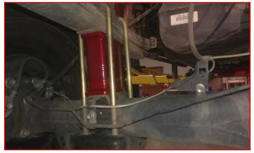
Install the provided u-bolts and nuts. Snug the u-bolt nuts but do not fully tighten at this time. Repeat steps for driver side.
