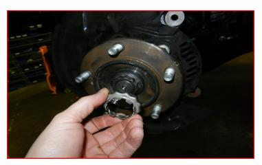
Remove the hub mounting bolts. Note: The bolts will not come off the hub.
