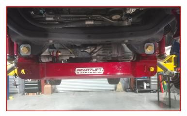
Install the ReadyLIFT passenger side diff mount to the front and rear cross member using 1/2" x 4" bolts, washers, and c-lock nuts. Do not tighten at this time. Carefully lower the differential down into the driver and passenger side mounts. Install using 1/2" x 4" bolts, washer, and c-lock nuts. Do not tighten at this time.
