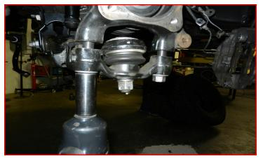
Remove the sway bar from the lower control arm and frame.
