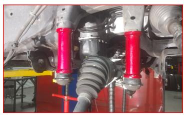
Install the bushing and sleeves into the ReadyLIFT differential mounts. Soapy water mixture will aid in installation. DO NOT use grease or WD40 as it will destroy the urethane.
