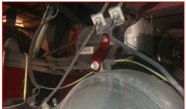
Install the parking brake brackets to the ReadyLIFT extensions (flat brackets) using  $5/16'' \times 1''$  bolts, washers, and c-lock nuts. Install completed assembly to the axle using factory hardware. Torque all hardware to 5 ft-lbs.
