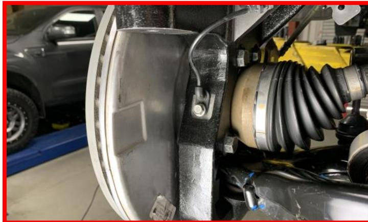
Torque the factory hardware to **80-in/lbs.**
