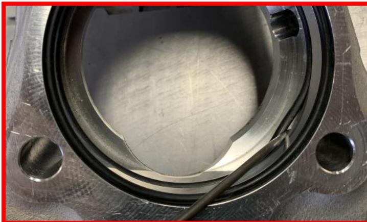
Install the o-rings from the factory knuckle into the replacement knuckle, take care when installing not to tear the o-rings.
