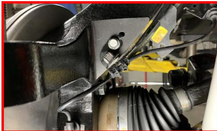
Torque the factory hardware to **80-in/lbs.**
