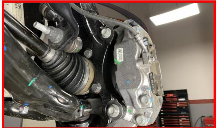
To gain the length needed to reach the ABS sensor mounting location it is necessary to remove the ABS sensor harness from the clip located passenger side inner fender.
