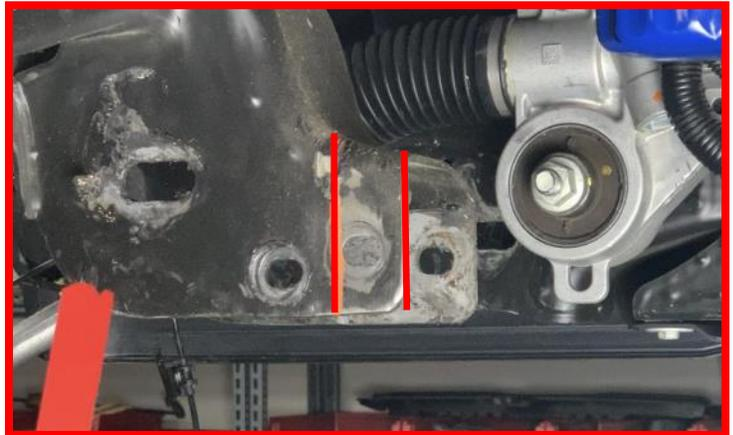
Measure from the pinion seal forward 6" and mark location. Measure from the outside of the fin inward approximately .375" and mark the location. Connect the two marks. Using an appropriate cutting tool cut away the material while following the marked line. Repeat steps for the bottom fin as well.
