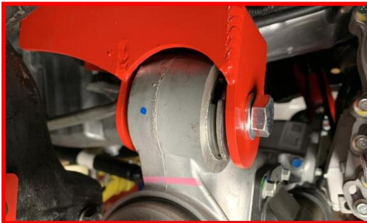
Tighten **driver differential drop bracket** hardware.
