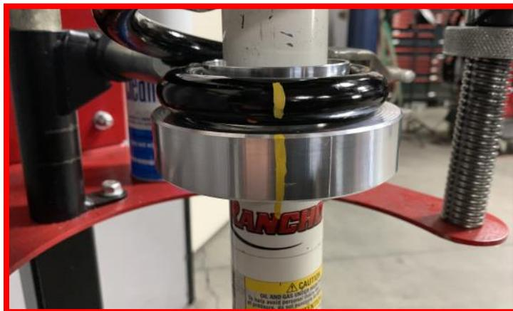
Install **front strut spacers** using factory nuts.
