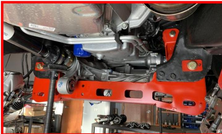
Install the (2) factory rear crossmember bolts and nuts and supplied cam block off plates, M18 bolt, washers and nut through the passenger side factory mount and replacement crossmember. Do not tighten hardware as this time.
