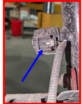
Unplug **line running from vehicle to ARC Sensor on strut assembly**.
