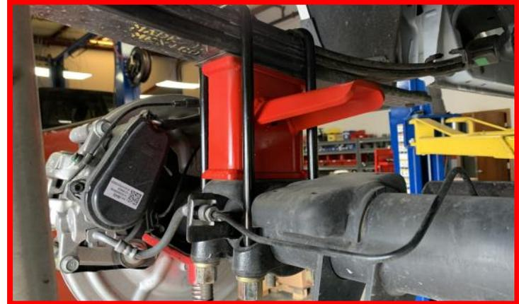
Install rear shock extensions into shock axle brackets.
