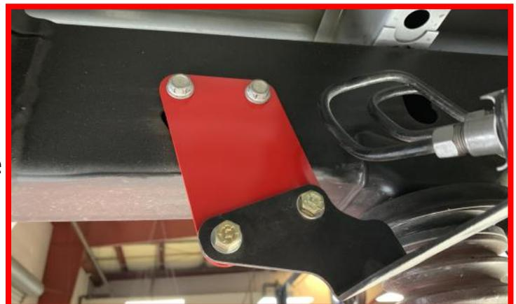
Install ABS harness drop bracket to the axle using the factory hardware.
