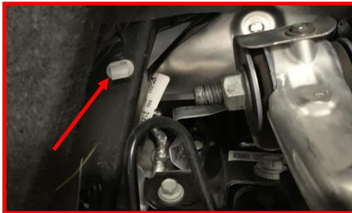
Route the ABS wire under the tie rod end boss on the knuckle and over the CV axle. Install **ABS sensor** into knuckle using the **factory hardware**.
