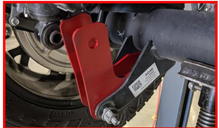
Install **factory fastener** between lower shock extension and lower shock axle bracket. Do not tighten at this time.
