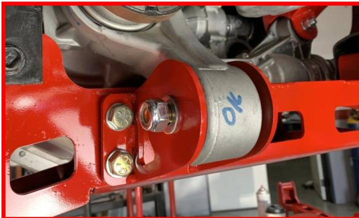
Tighten **passenger differential drop bracket** hardware.
