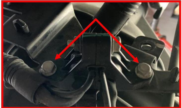
Support the axle with a suitable jack. Remove both **driver and passenger shock lower bolts** from vehicle and retain factory hardware.
