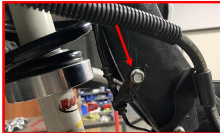
Torque the factory hardware to **80-in/lbs.**
