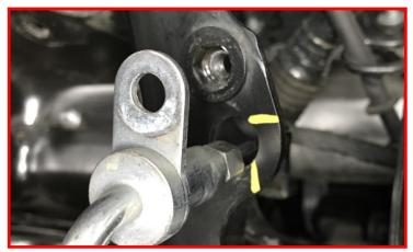
Remove brake line from factory mounting area.
