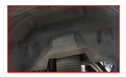
Release the air pressure in the rear air bags by loosening the line at the top of the air bag.
