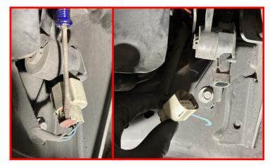
Remove the ride height sensor link from the control arm using a small pry bar or similar tool.
