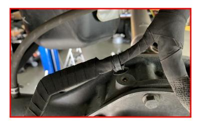
Remove the harness retaining clip from the stud on the rear differential cover.
