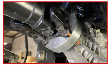
NOTE: Due to variation in vehicle models, you may need to trim the plastic bracket on the side of the transmission due to contact with the driveshaft.
