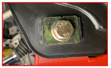
Install rear crossmember using the supplied cam block off plates, M18 bolts, washers, and nuts.
