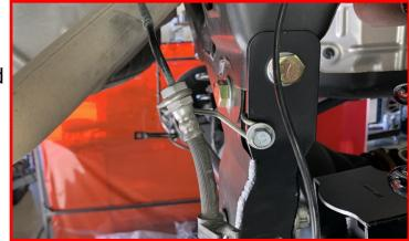
Install the ABS retaining clip into the factory brake line bracket location.
