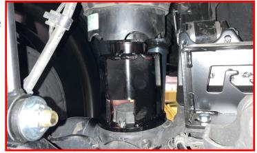
Install the air line fitting at the top of the bag.
