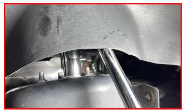
Remove the outer tie rod end nut.
