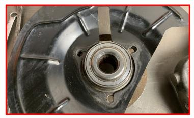
Install rotor dust shield and hub assembly into replacement knuckle using the (3) factory hub bolts and thread locker.
