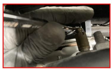
Loosen the three top air strut nuts but do not remove at this time.
