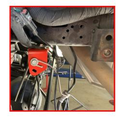
While gently pulling down on the brake line install the factory brake line bracket onto the rear track bar bracket using the factory hardware and supplied M8 nut and washer.
