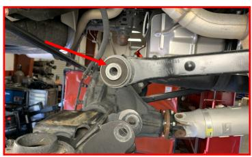
Install the supplied passenger upper control arm bracket to the axle using the supplied M10 x 35mm bolts, nuts and washers. Do not tighten at this time.
