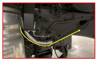
Install the completed air strut assembly using the supplied M10 serrated flange nut.
