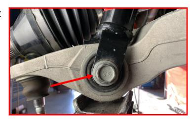
Swing lower control arm down and out of the way. Remove the (3) top strut nuts and carefully remove the strut from the vehicle.
