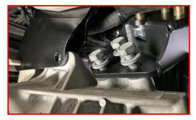
Install the provided M12 x 60mm bolt and washers through the passenger side rear differential drop bracket, the differential housing, then the passenger side front differential drop bracket.
