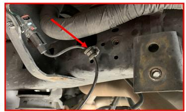
Remove the harness retaining clip from the top of the rear differential.
