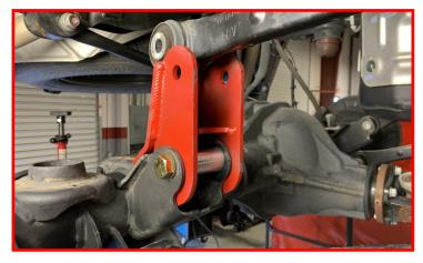
Install the supplied M8 bolt and washer through the upper control arm bracket and into the axle. Do not tighten at this time.
