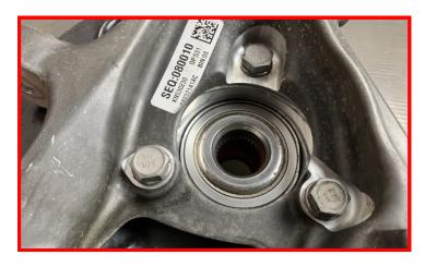
Remove hub assembly from factory knuckle.
