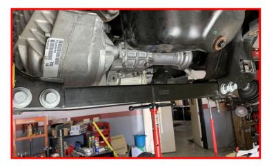
Mark the driveshaft to pinion flange location. Remove the front driveshaft hardware from the flange. Let driveline hang out of the way. Discard the factory hardware.
