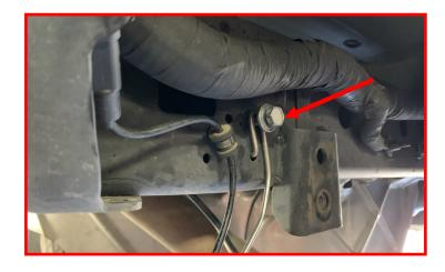
Remove the driver ABS retaining clip at the frame rail.
