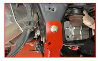
Note the location and orientation of track bar bracket nut plate.
