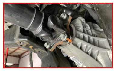
Unplug the differential shift actuator. Ensure all clips are removed and clear of the differential.
