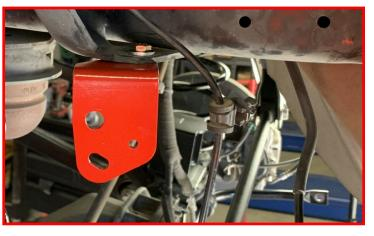
While gently pulling down on the brake line, install the factory brake line bracket onto the driver rear brake line bracket using the factory hardware and supplied M8 nut and washer.
