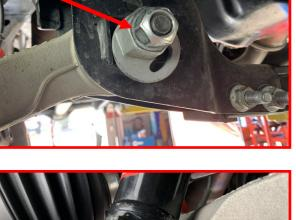
Remove the lower control arm from the frame. Be sure to retain factory alignment cam bolts, cams and nuts.
