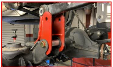
Install the supplied M8 bolt and washer through the upper control arm bracket and into the axle. Do not tighten at this time.
