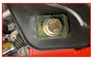
Install rear crossmember using the supplied cam block off plates, M18 bolts, washers, and nuts.
