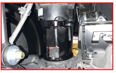
Install the air line fitting at the top of the bag.
