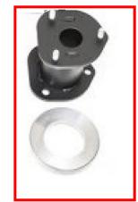
Locate the top strut extension and install using the factory hardware.
