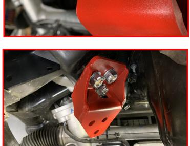
Raise differential into place. Be sure to use a helper to aid in the installation process. With the differential in place, install the provided M12 x 60mm bolt, washers and nut through the driver side inner differential drop bracket, the diff drop spacer, the differential housing, then the driver side outer differential drop bracket.
