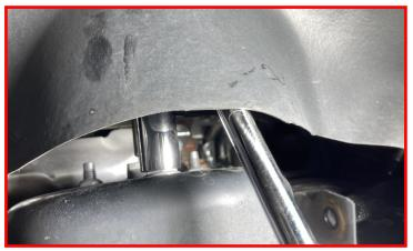
Remove the outer tie rod end nut.
