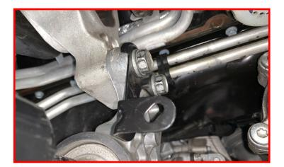
Remove the (3) driver side rear differential mounting hardware. Retain the factory hardware.
