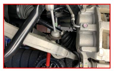
Using a couple wire ties, secure the ABS sensor harness to the brake line.
