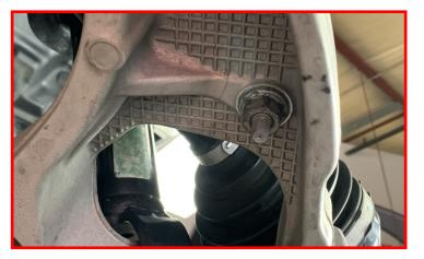
Remove (4) sway bar mounting bolts from the frame and retain the factory hardware. Remove sway bar from the vehicle.
