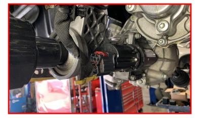
Install the top harness retaining clip into the shift solenoid harness bracket.
