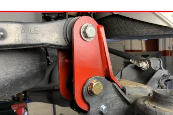
Attach the track bar bracket support tab to the factory track bar mount using the track bar bracket nut plate, the supplied M12 x 35mm bolt and washers and tread locker. Tighten all mounting hardware at this time.
