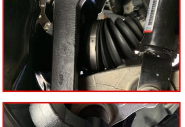
Install the opposite side ABS wire bracket on the inside of the knuckle using the factory hardware (i.e. Driver will be installed on passenger side).
