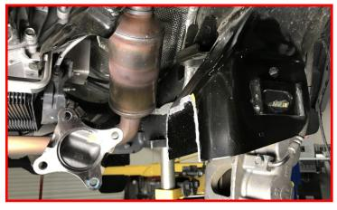
\*\*\*Parts shown in red for picture clarification only\*\*\* Install the driver side differential drops
