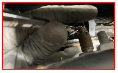
Loosen the three top air strut nuts but do not remove at this time.
