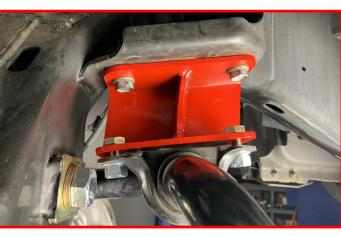
Install the sway bar drop link into the lower control arm using factory nut.
