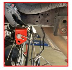
Install the ABS retaining clip into the driver rear brake line bracket in the bottom hole. Tighten the bracket at this time.
